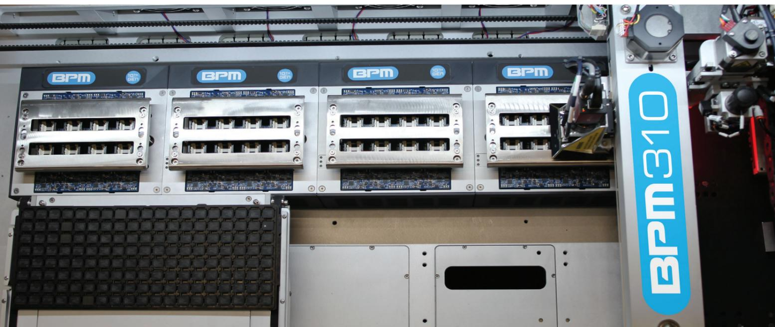
The new BPM310 is the latest 10th Generation Automated Programmer from BPM Microsystems. It features up to 6 fully universal programming sites with up to 48 sockets, producing the fastest programming times in the smallest footprint while offering advanced features such as WhisperTech™, BPM.NCRYPT, and on-the-fly vision alignment. Unlike other products in
